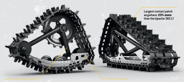
Efficient frame and rail design ensures weight is evenly distributed on snow
